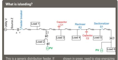
shown in green, need to stop energizing the isolated part of the grid. If they don't, that section of the grid that's still energized is an unintentional island.
